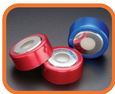
BiMetal Seals. Coloured Outer surface is Aluminium making them easy to crimp but still magnetic due to inner tin surface.
