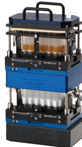
Two 48-Positions Blue SiliCycle MiniBlocks with Transfer Adapter and Positive Pressure Manifold
