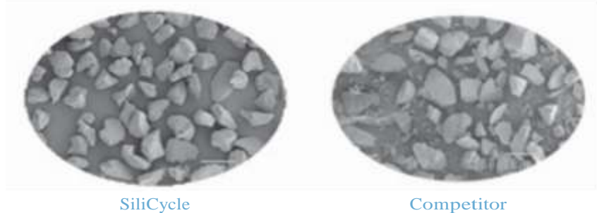
Scanning Electron Microscopy (SEM) Comparison of Two Silica Gels 40 - 63 \mu\text{m} , 60 \text{\AA}
