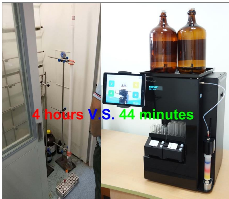
Figure 3. The comparison of manual chromatography method with automatic purification method.
