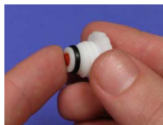
FIG. 6 INSERTING NEW SEPTUM
