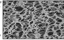
PES (polyethersulfone) filters are inert which provide extremely low extractable levels in critical sterilization applications such as protein and enzyme filtrations,
